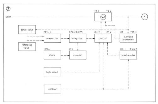
The low speed is automatically stabilised so as to obtain a constant speed level under varying load conditions. This is done in the following manner:
