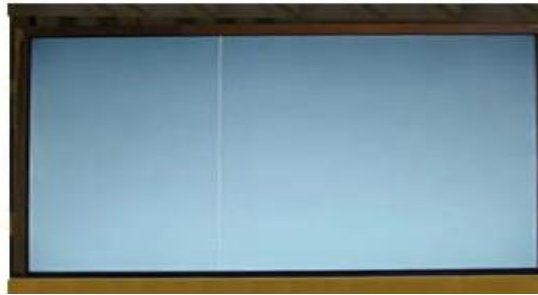
Vertical Line Source TAB IC Defect
