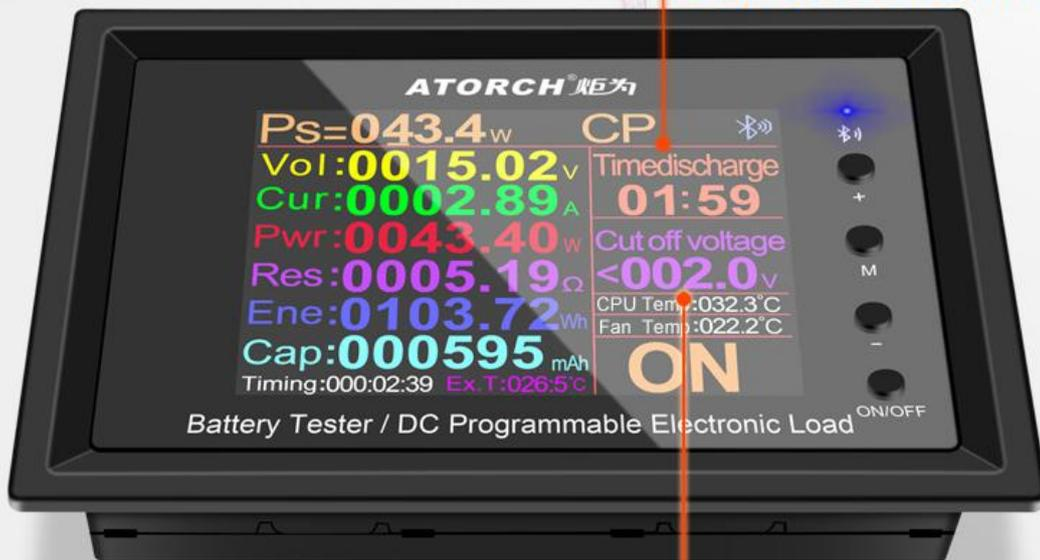
Can be set Cut-off discharge voltage
