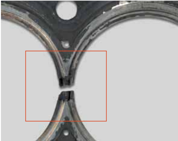
▲ Broken web caused by high component dynamics
