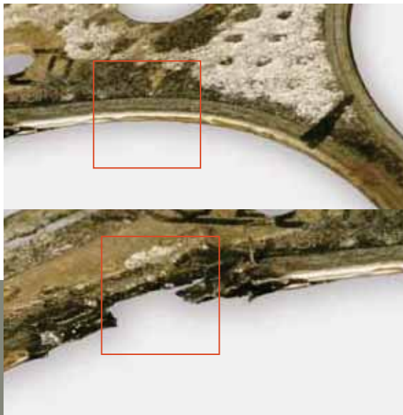
▲ Indentation and crushing due to pre-ignition – with and without blowby.
