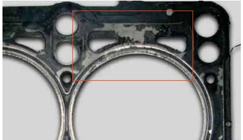
▲ Elastomer coating damaged by overheating
