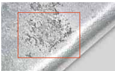
▲ Gasket damage due to dirt and foreign objects.
