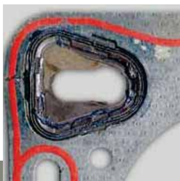
▲ Tearing and breakage of the composite material, and damaged Viton element due to incorrect application of additional sealing compound.
