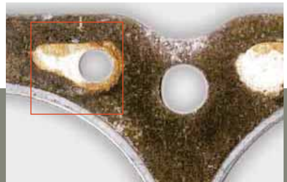
▲ Swelling of composite cylinder-head gaskets due to overheating with steam generation.
