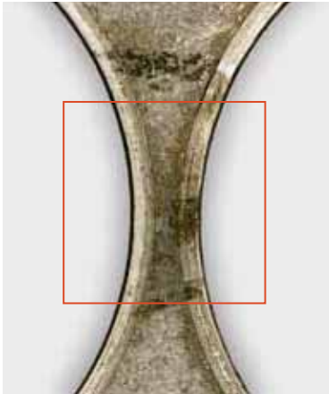
▲ Gas leakage with local blackening of the fire ring bead.
