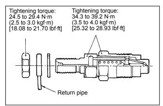
Figure 99 Assembling the nozzle
