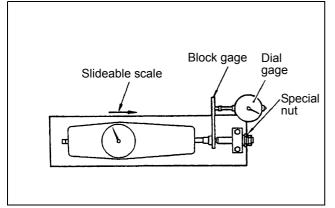
Figure 107 Inspecting torque spring
