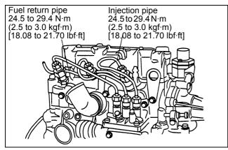
Figure 102 Installing injection pipe
