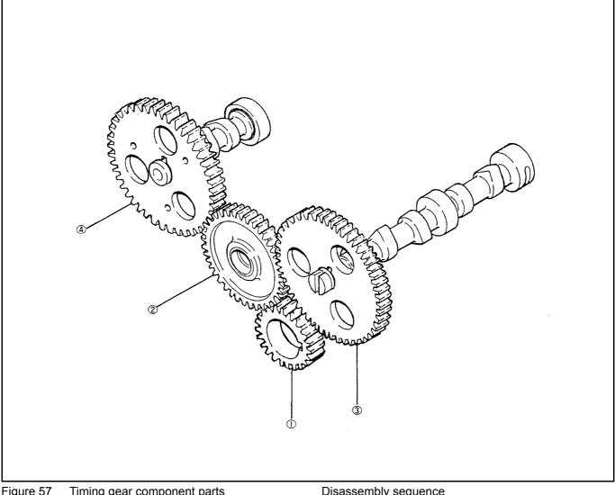
Figure 57 Timing gear component parts **Disassembly sequence**
