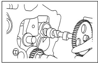
Figure 59 Removing camshaft gear
