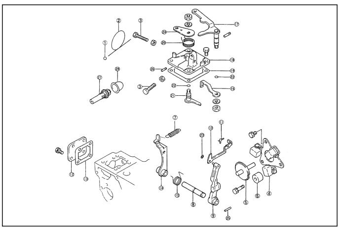
Figure 103 Governor system component parts
