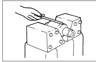
Figure 129 Checking armature coil
