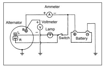
Figure 136 Checking for output
