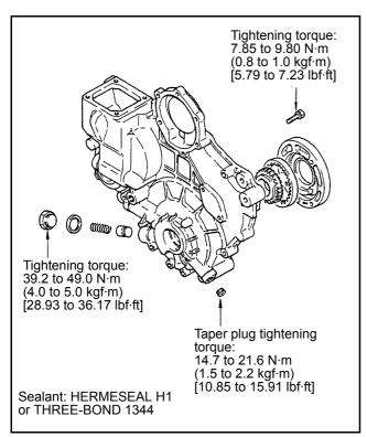
Figure 55 Gear case assembly
