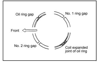
Figure 75 Proper arrangement of ring gaps
