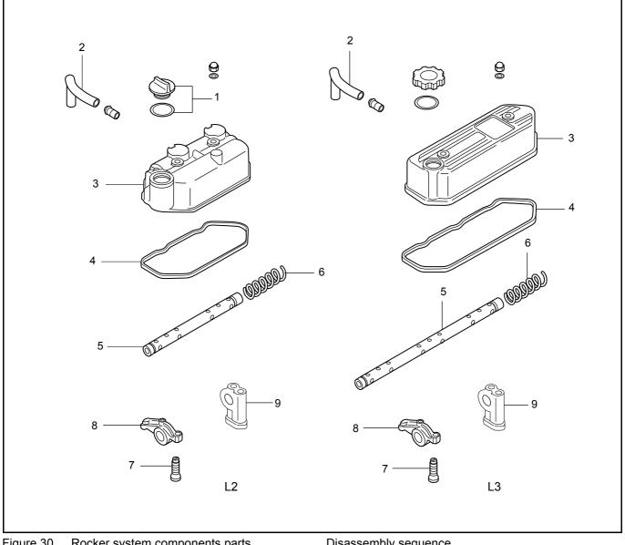
Figure 30 Rocker system components parts
