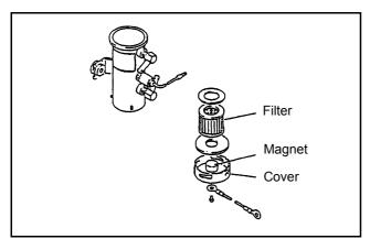
Figure 16 Plunger type (common) fuel pump
