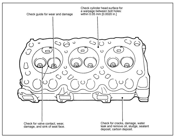
Figure 37 Inspection of cylinder head
