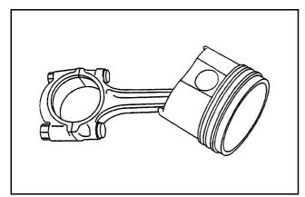
Figure 76 Fitting cap to connecting rod
