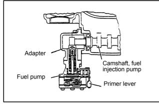
Figure 19 Mechanical type fuel pump
