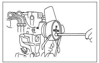
Figure 113 Removing water pump
