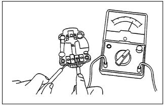
Figure 139 Checking diodes
