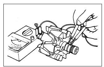
Figure 140 Checking field coil for continuity
