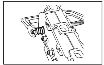
Figure 36 Removing valves
