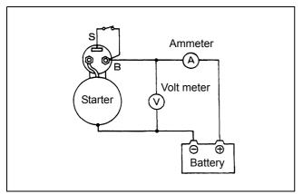
Figure 121 No-load test
