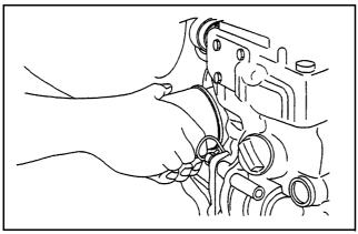
Figure 88 Installing oil filter
