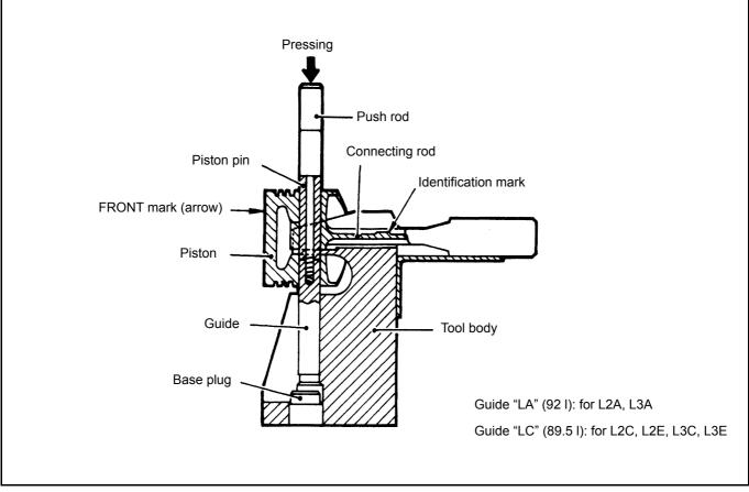
Figure 73 Reassembling piston pin
