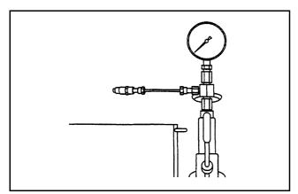
Figure 25 Testing injection start pressure
