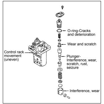
Figure 94 Inspection of injection pump
