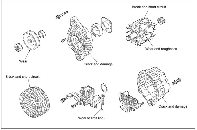
Figure 138 Inspection of alternator
