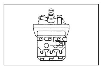
Figure 3 Injection pump
