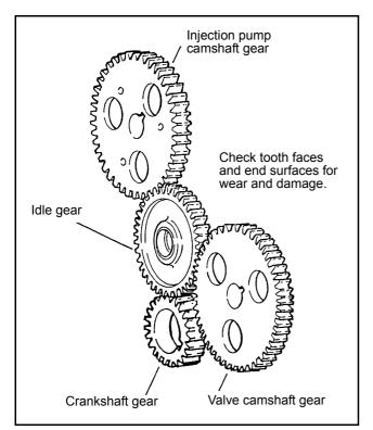
Figure 60 Inspecting timing gears
