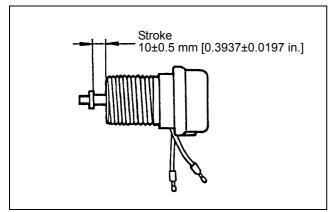
Figure 150 Fuel cutoff solenoid (ETS type)
