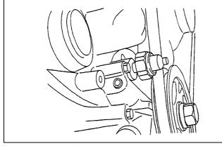
Figure 89 Installing pressure switch
