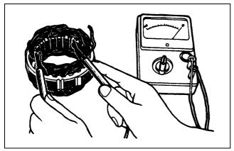
Figure 142 Checking stator coil for continuity
