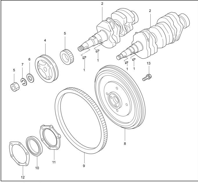
Figure 77 Crankshaft component parts
