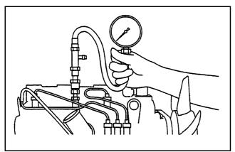
Figure 29 Testing compression pressure
