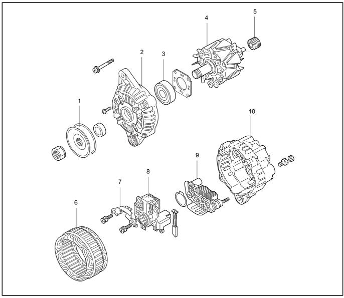
Figure 133 Alternator component parts
