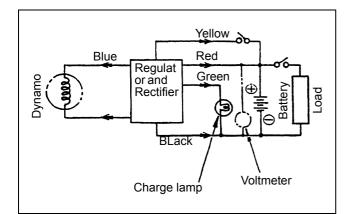
Figure 146 Measuring voltage across battery terminals
