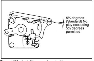
Figure 109 Installing speed control lever
