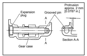
Figure 54 Reassembling governor shaft
