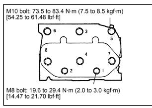
Figure 8 Cylinder head bolt tightening sequence (L2)
