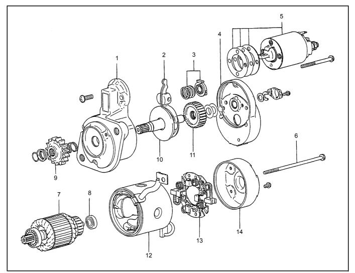
Figure 119 Starter component parts
