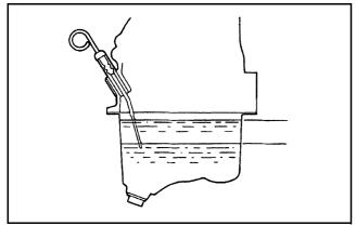
Figure 5 Checking oil level
