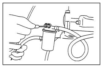
Figure 13 Fuel filter air bleeding
