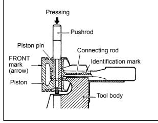
Figure 68 Removing piston pin
