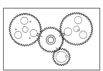
Figure 61 Timing gears in alignment
