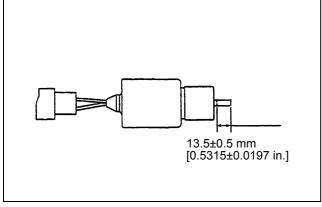
Figure 152 Fuel cutoff solenoid (ETR type)
