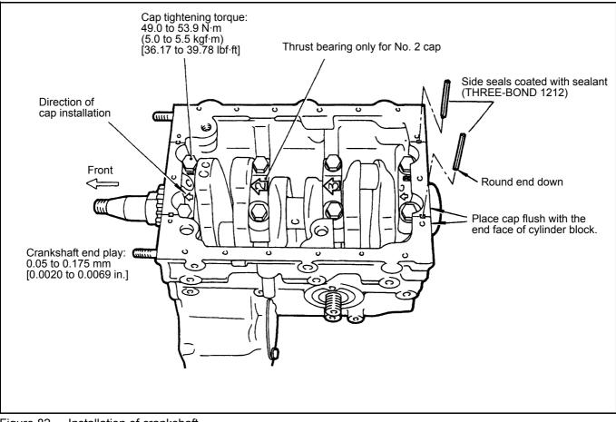
Figure 82 Installation of crankshaft
