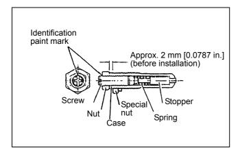
Figure 105 Assembling torque spring set
