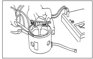
Figure 131 Checking field coil
