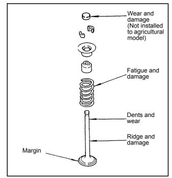
Figure 45 Inspection of valve and valve spring
