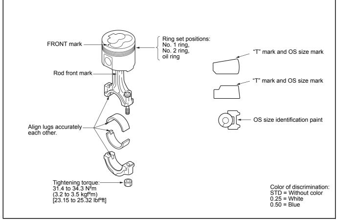
Figure 74 Reassembly of piston rings and connecting rod cap
