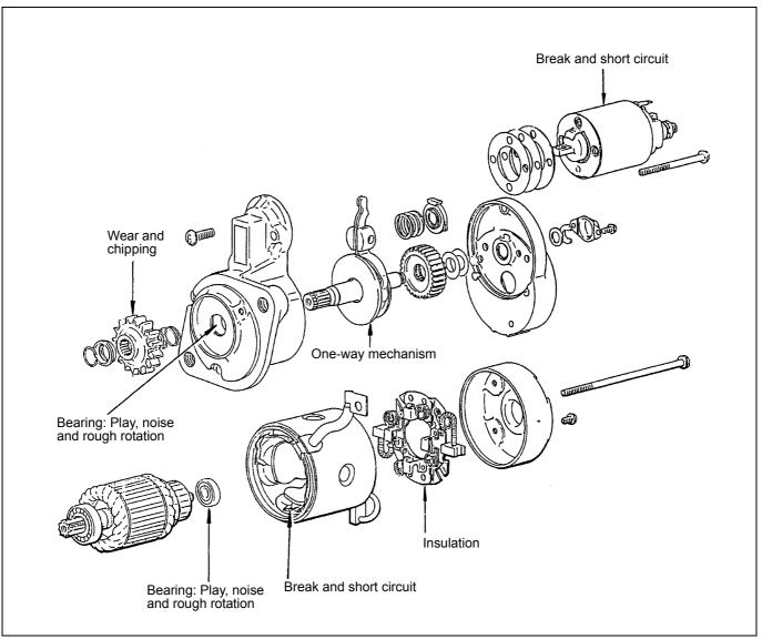
Figure 127 Inspecting starter
