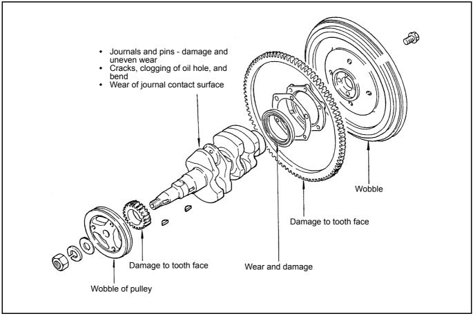
Figure 79 Inspection of crankshaft and flywheel
