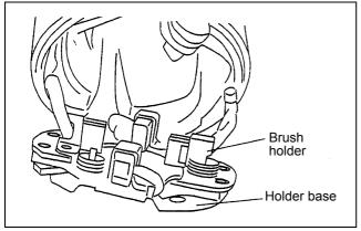
Figure 130 Checking brush holders
