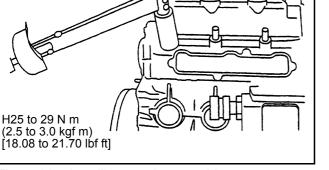
Figure 26 Installing nozzle assembly
