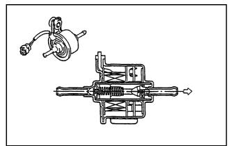
Figure 17 Plunger type (compact) fuel pump
