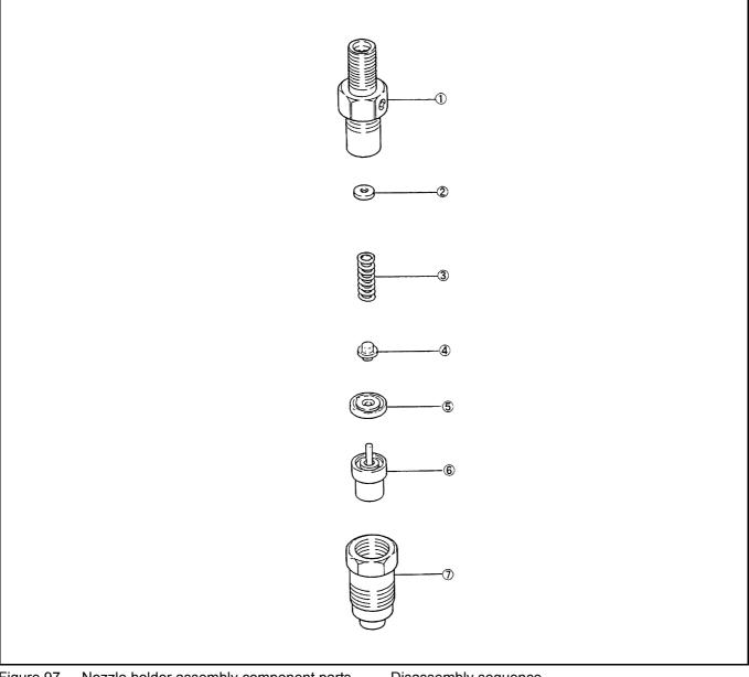
Figure 97 Nozzle holder assembly component parts
