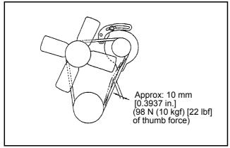
Figure 12 Adjusting fan belt tension
