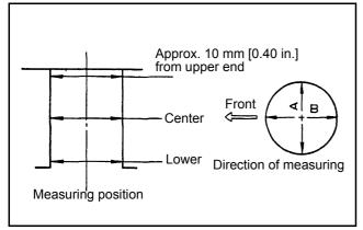
Figure 85 Cylinder bore measuring positions
