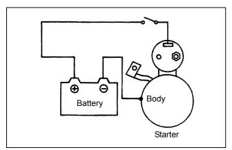
Figure 123 Holding test
