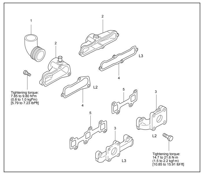
Figure 49 Manifold component parts
