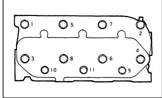
Figure 35 Sequence for loosening cylinder head bolts (L3)
