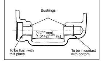
Figure 52 Press-fitting governor shaft bushing
