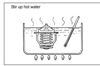
Figure 115 Inspecting thermostat
