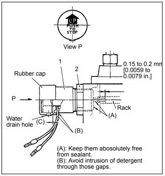
Figure 151 Solenoid installation
