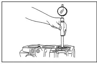
Figure 84 Measuring cylinder bore
