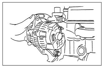
Figure 137 Removing alternator
