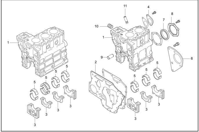
Figure 83 Cylinder block component parts
