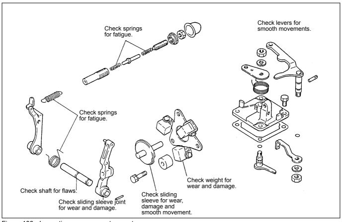
Figure 108 Inspection governor system parts
