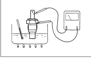
Figure 116 Inspecting temperature gage unit
