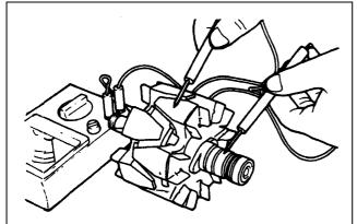
Figure 141 Checking field coil for insulation
