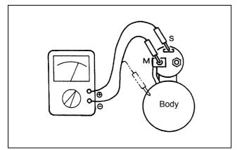
Figure 128 Checking magnetic switch
