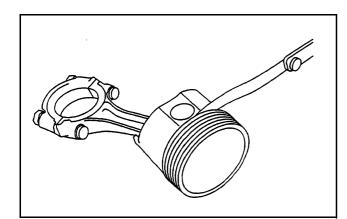
Figure 71 Measuring ring side clearance
