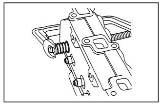
Figure 44 Removing valve and valve spring
