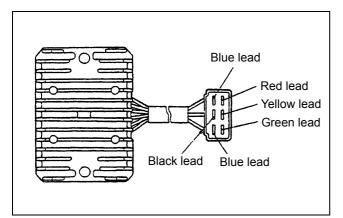
Figure 147 Lead outlet coupler
