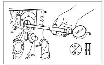
Figure 81 Measuring main bearing I. D.
