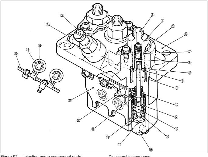
Figure 92 Injection pump component parts
