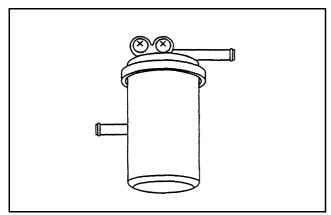
Figure 15 Cartridge type filter
