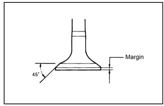
Figure 47 Inspecting valve
