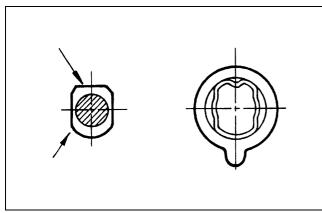
Figure 95 Direction of reassembly of plunger
