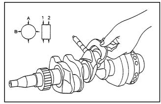
Figure 80 Measuring ring gap
