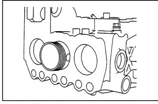
Figure 67 Removing connecting rod and piston
