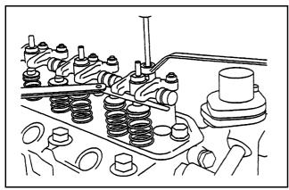
Figure 10 Adjusting valve clearance
