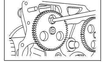
Figure 63 Removing injection pump camshaft
