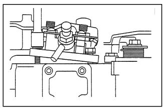
Figure 23 Removing injection pump
