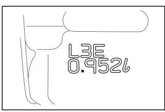
Figure 1 Engine model and cylinder volume
