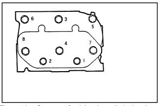
Figure 41 Sequence for tightening cylinder head bolts (L2)
