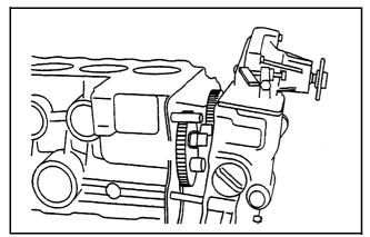
Figure 56 Installing gear case assembly
