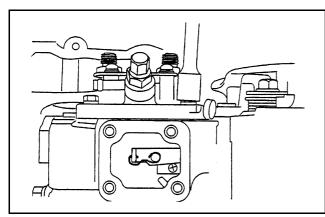
Figure 93 Removing injection pump
