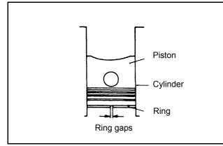
Figure 70 Measuring ring gap
