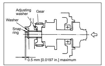
Figure 132 Adjusting pinion shaft end play
