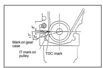
Figure 21 Injection timing mark
