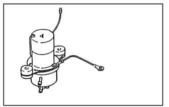
Figure 18 Diaphragm type fuel pump
