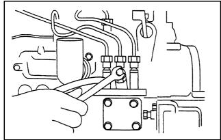
Figure 14 Fuel injection pump air bleeding
