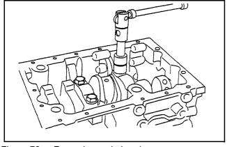
Figure 78 Removing main bearing cap
