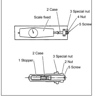
Figure 106 Setting of torque spring
