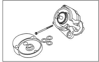
Figure 126 Removing reduction gear
