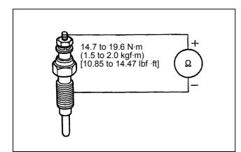
Figure 148 Checking glow plug
