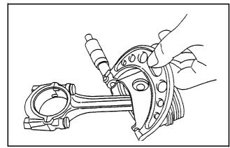
Figure 86 Measuring piston diameter
