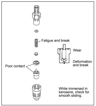
Figure 98 Inspecting nozzle
