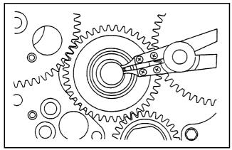
Figure 58 Removing idle gear
