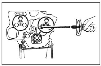
Figure 65 Installing valve camshaft
