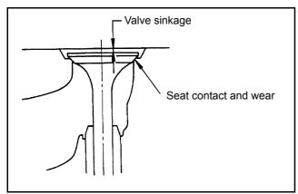
Figure 39 Checking valve sinkage
