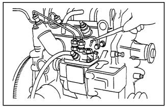
Figure 20 Removing delivery valve
