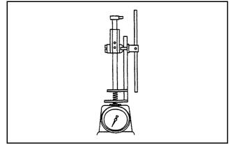
Figure 46 Valve spring tester
