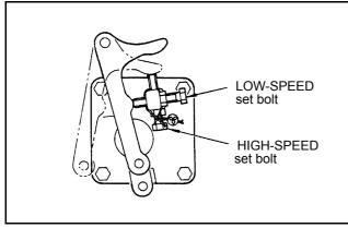
Figure 24 HIGH-SPEED and LOW-SPEED set bolts
