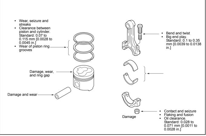
Figure 69 Inspection of piston and connecting rod
