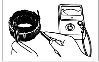
Figure 143 Checking stator coil for insulation
