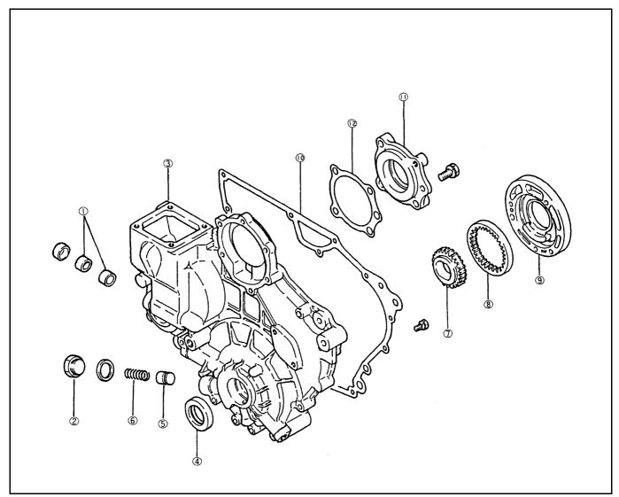
Figure 50 Gear case component parts
