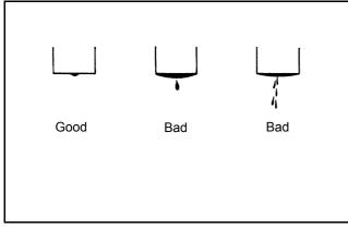
Figure 28 After-spilling
