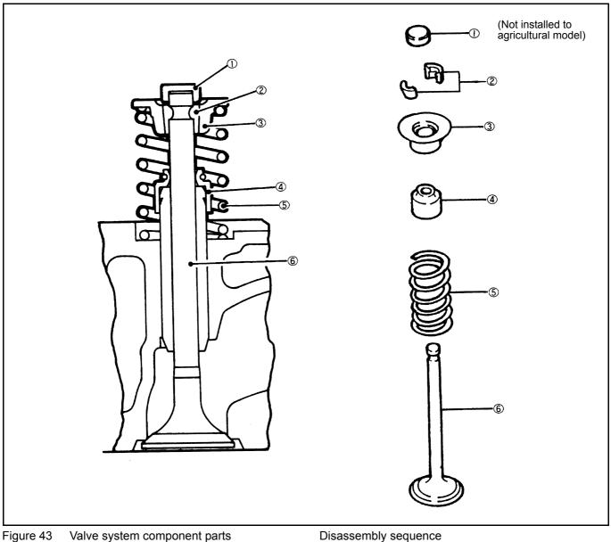
Valve system component parts
