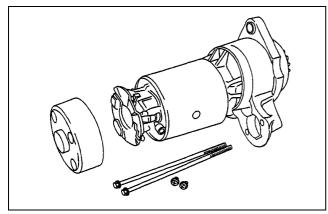
Figure 125 Removing brush holder assembly
