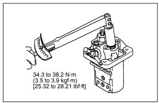
Figure 96 Installation of delivery valve holder
