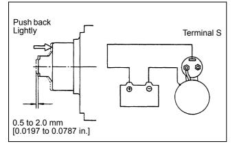
Figure 120 Inspecting pinion gap
