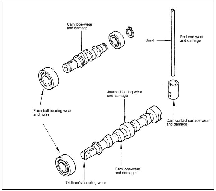
Figure 64 Inspection of camshafts
