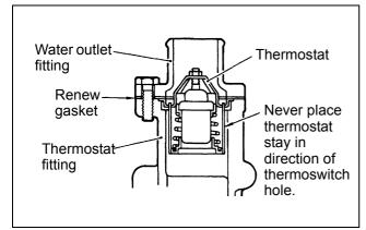
Figure 114 Installing thermostat
