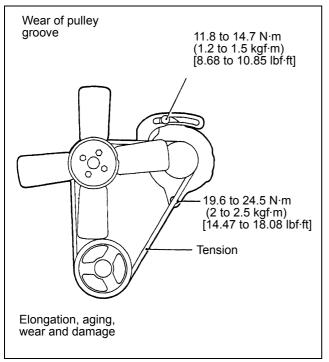
Figure 111 Inspecting fan belt
