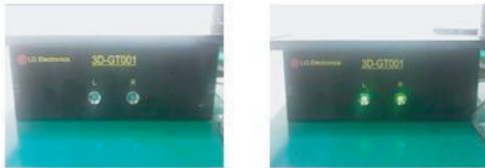
<IR Tester Lamp turned off(NG)> <IR Tester Lamp turned on(OK)>
