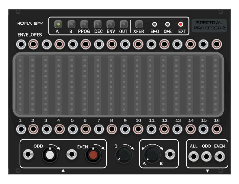
The spectral processor is a 16-channel bandpass filter, it can work as a real-time performance filter, a programmable compound equaliser and even as a spectrum transferring vocoder.
