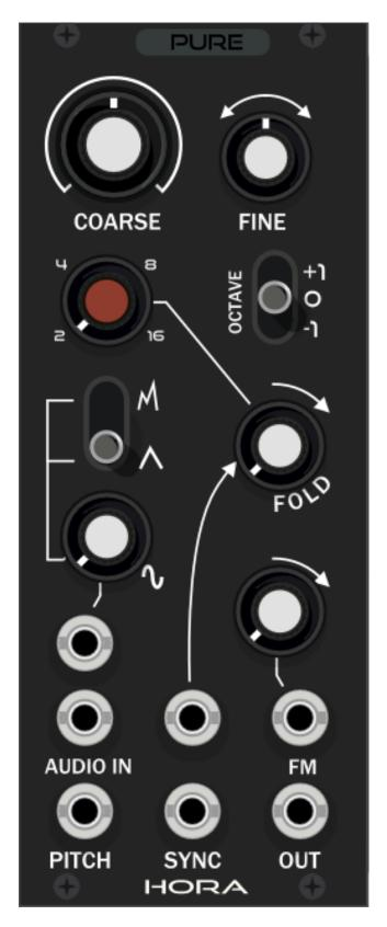
Pure VCO is a voltage-controlled oscillator that generates complex waveforms. The core wave can be morphed from sine to triangle and then is folded in a specific way to give harmonics without sharp edges in the folded waveform.
