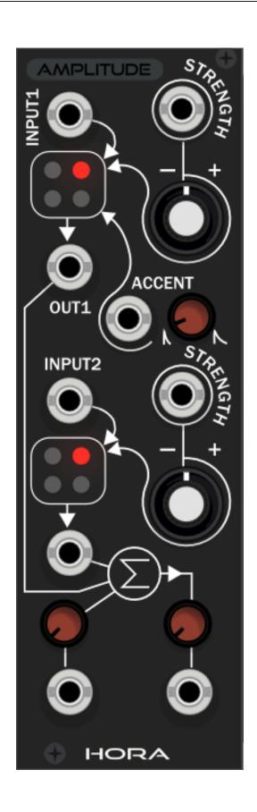
Amplitude is made of two VCAs that offer voltage-controlled attenuation - inversion (called strength). The two VCAs outputs and an auxiliary input are sent to a mixer. The aux input has a dedicated attenuator.
