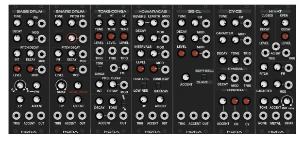
The Hora ANALOG DRUMS collection is a set of analog modelled percussion voices. While the modules are inspired by the famous 808 vintage drum machine, they also offer an in-depth control of the sound, some additional features, and CV control over many parameters.
