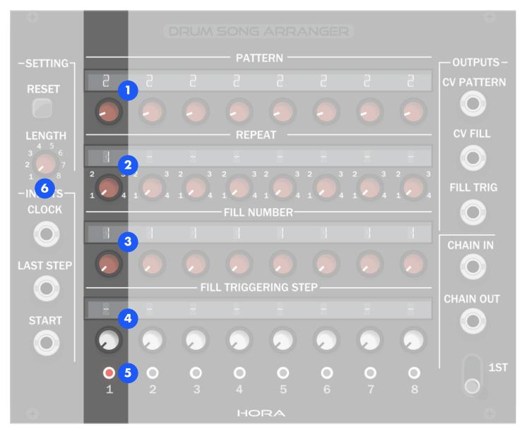
When a pattern arrives at its end, the drum sequencer sends a signal through the "last step" connexion. The drum song arranger then repeats the section if specified. If not, it will switch to the next section.
