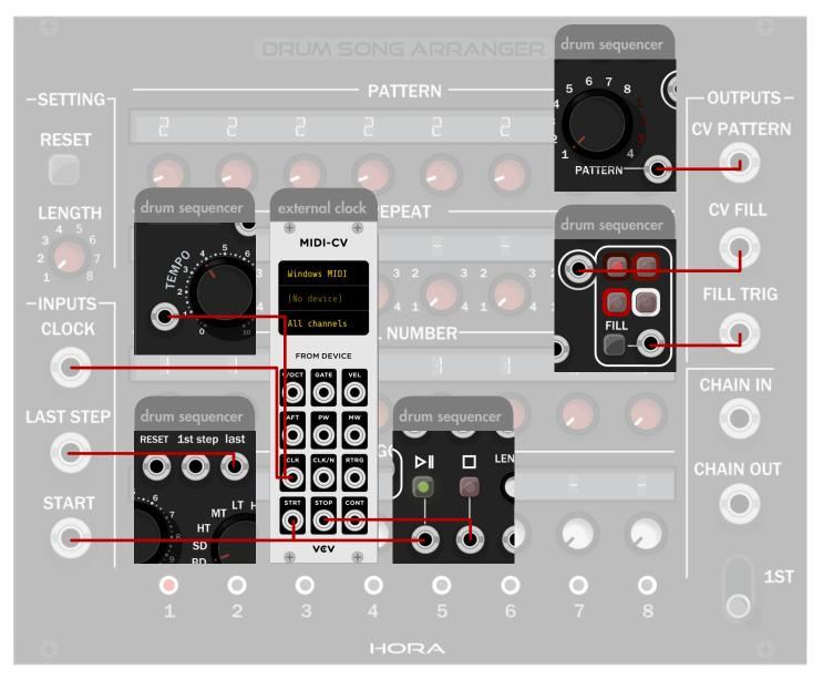
The drum song arranger is made to control the pattern selection, fill selection and fill triggering of the Drum Sequencer. Therefore, these outputs have to be correctly connected.
