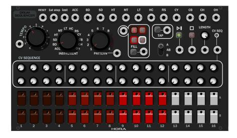
This plugin is designed to sequence the analog drums modules but can be used to trig any other drum module, envelopes, sampler module,...
