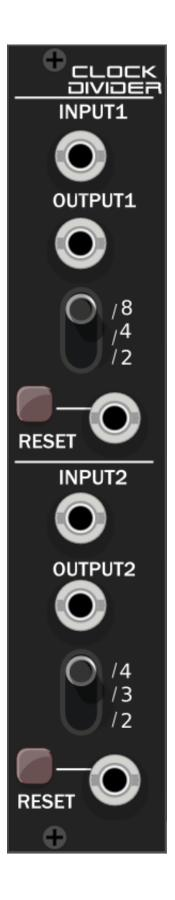
The Hora Clock divider is a utility module with two gate dividers. The division can be set in different ways using the 3 position switch. The count can be reset by the push button or the gate input.
