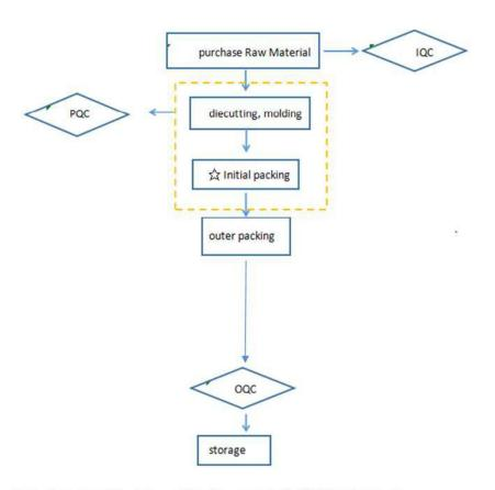
NOTE: in process of diecutting, molding, there is in the 100,000 class cleaning room the process marked with ▲ is the special process. marked with ☆ this is the Key process
