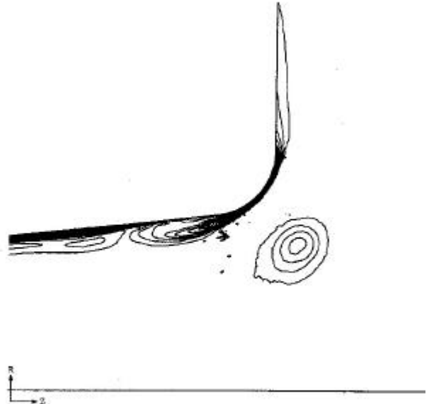
(c) time t=13 ms (maximum vorticity in vortex 0.5417E4 radians/s)
