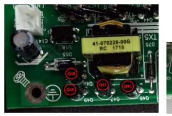
The Q46and Q48 are 11-300012-00G (TR 2A 50V NPN TO-92) The Q47and Q49 are 11-300005-00G (TR 2A 50V PNP TO-92NL)
