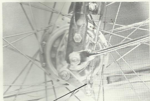
Left side front brake coarse adjustment
