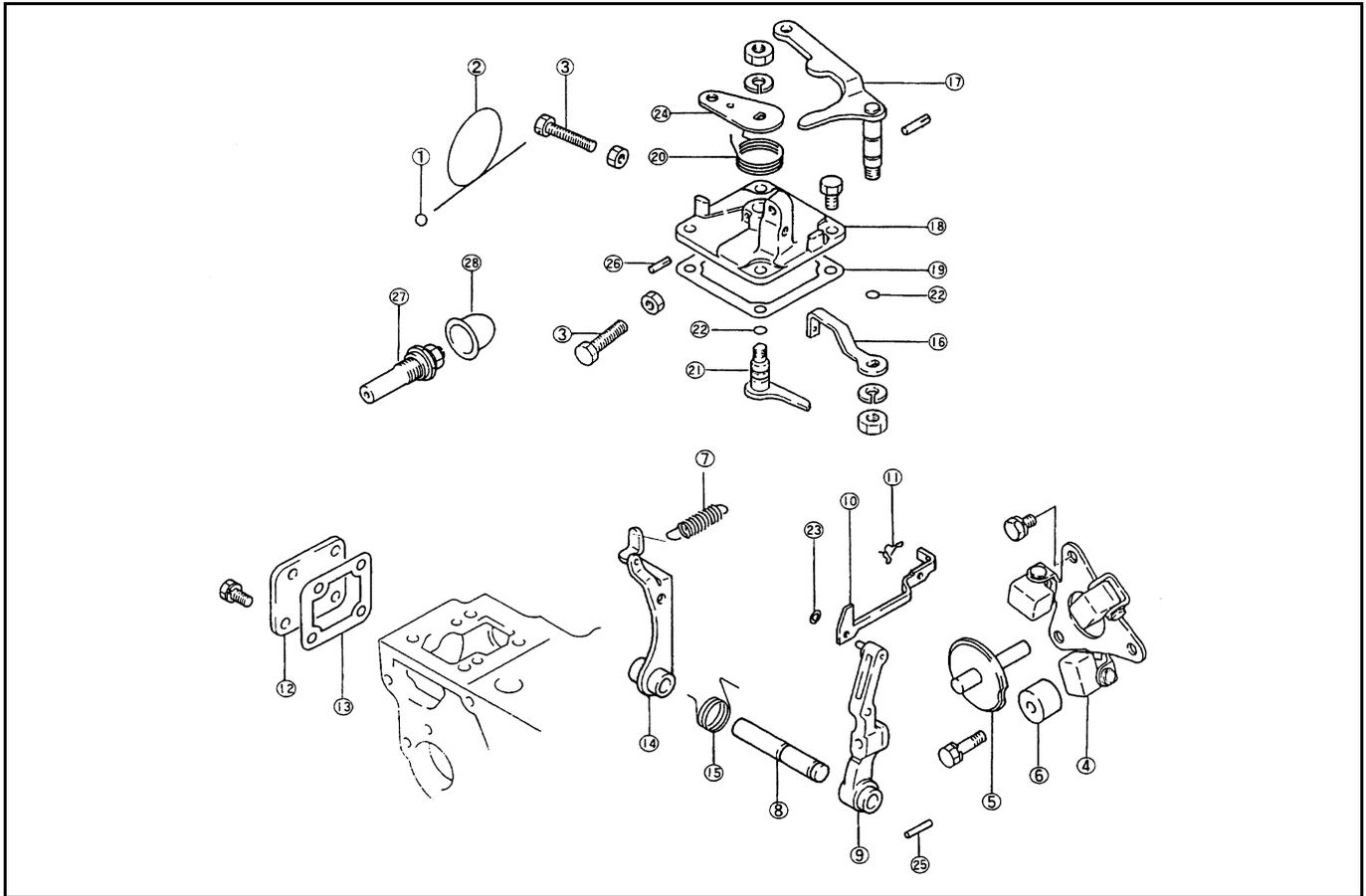
Figure 103 Governor system component parts
