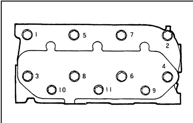
Figure 35 Sequence for loosening cylinder head bolts (L3)
