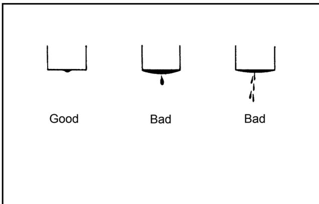
Figure 28 After-spilling
