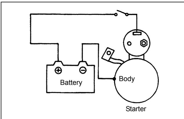
Figure 123 Holding test
