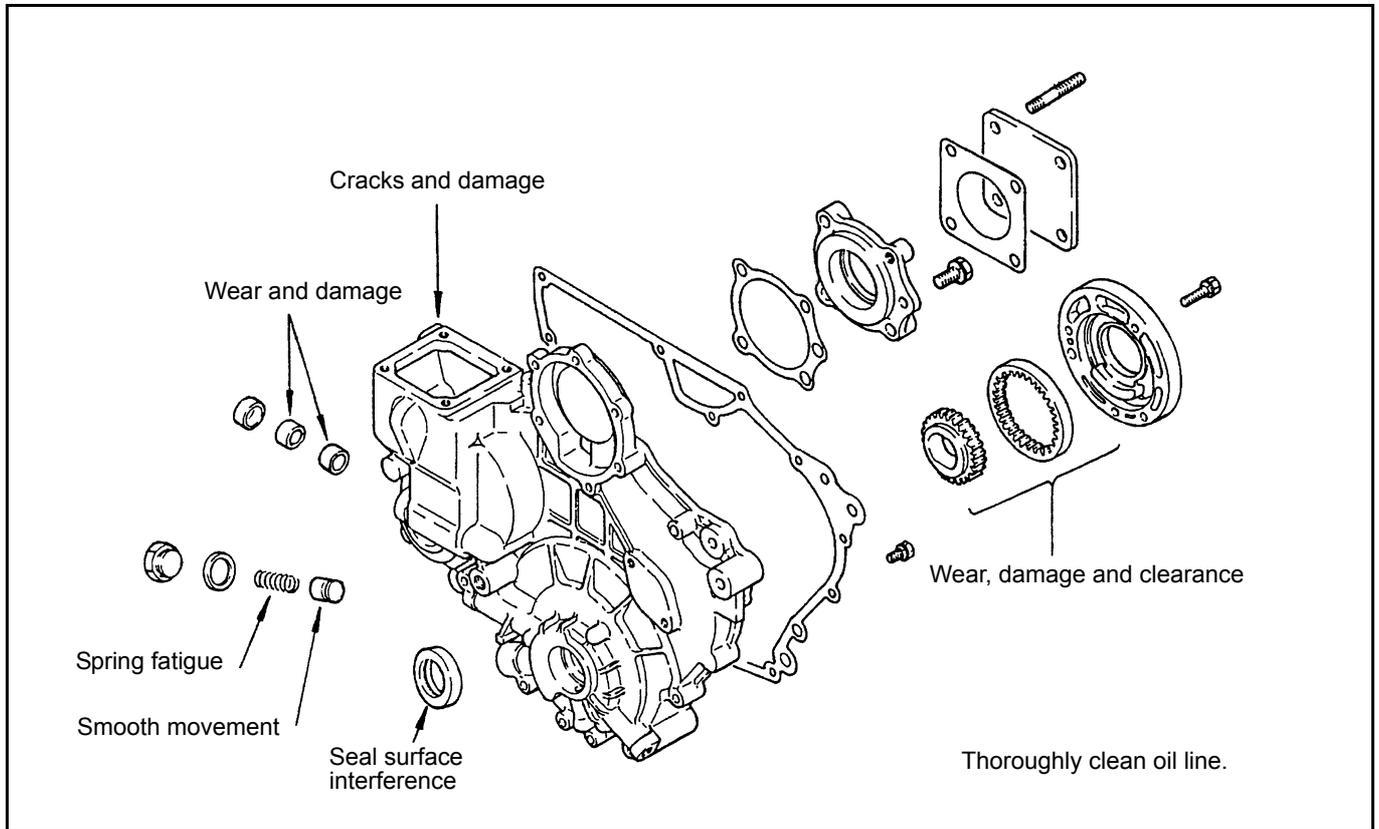
Figure 51 Inspection of gear case and oil pump
