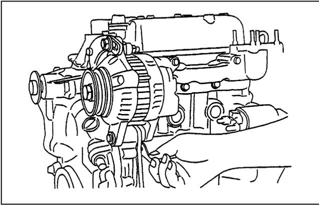
Figure 145 Inserting spacer
