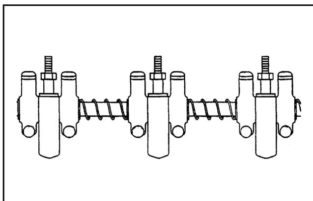
Figure 32 Inspecting rocker shaft and rocker arms
