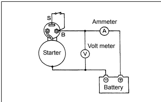
Figure 121 No-load test
