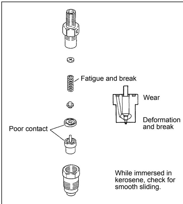
Figure 98 Inspecting nozzle
