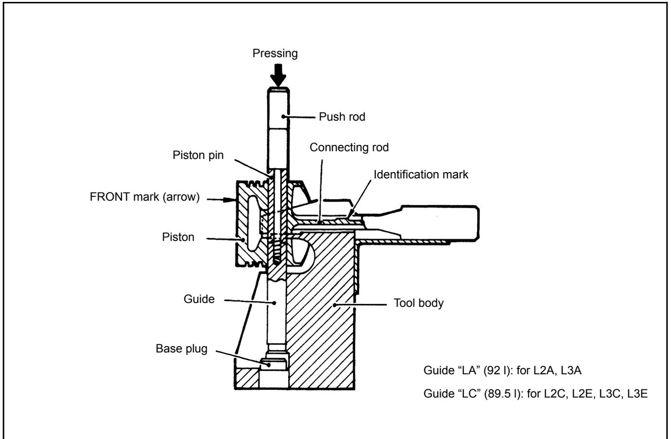
Figure 73 Reassembling piston pin
