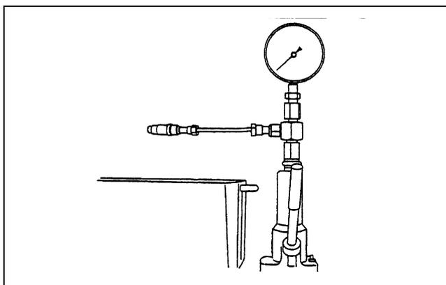
Figure 100 Testing nozzle
