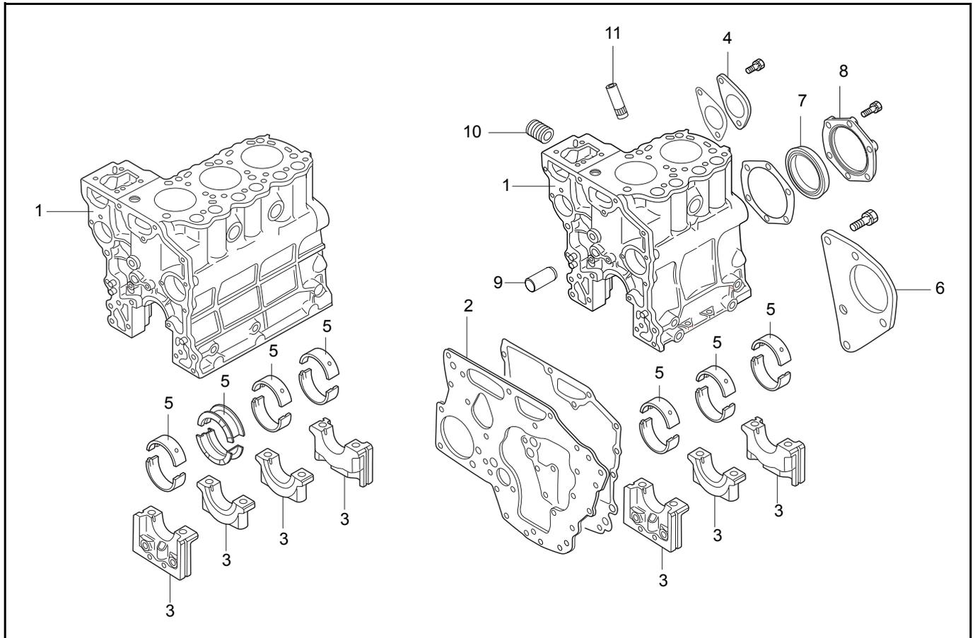
Figure 83 Cylinder block component parts
