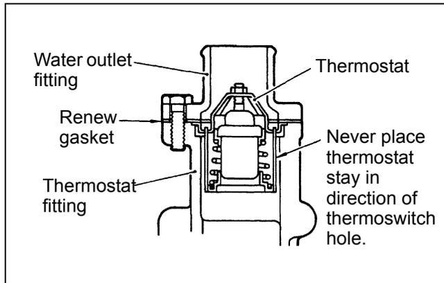
Figure 114 Installing thermostat
