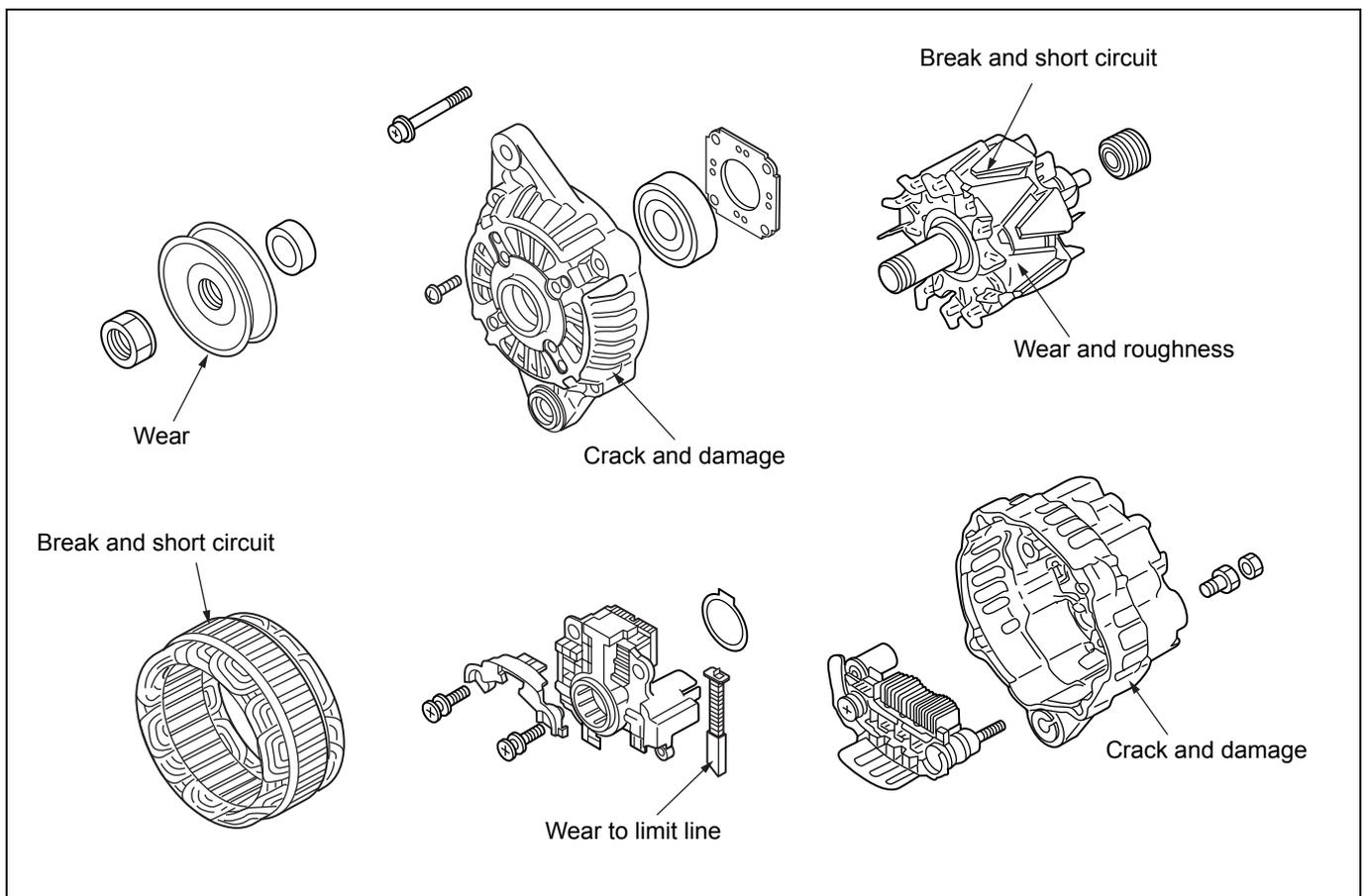
Figure 138 Inspection of alternator
