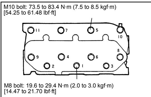
Figure 9 Cylinder head bolt tightening sequence (L3)
