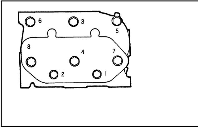
Figure 41 Sequence for tightening cylinder head bolts (L2)
