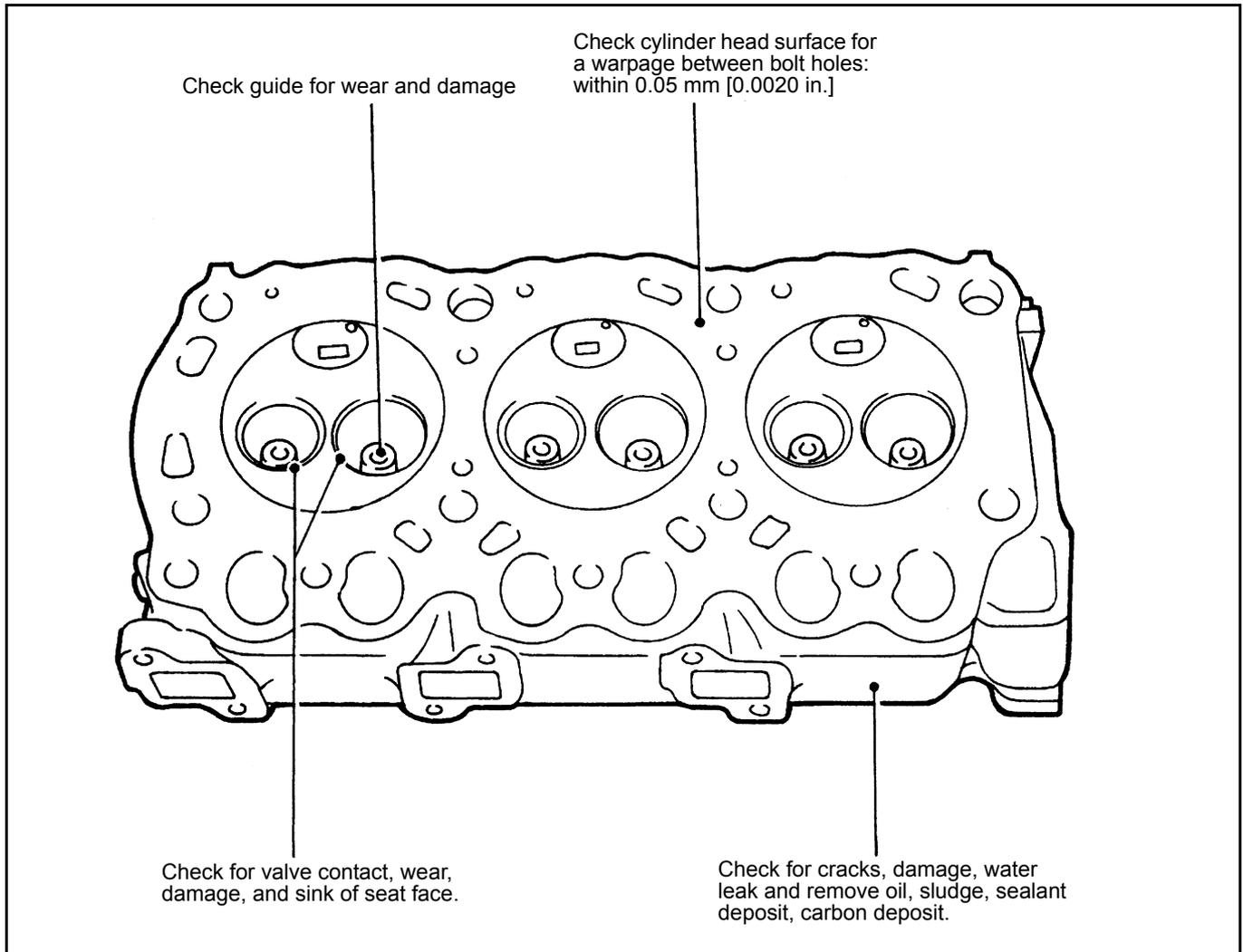
Figure 37 Inspection of cylinder head
