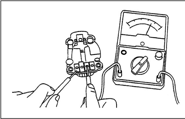
Figure 139 Checking diodes
