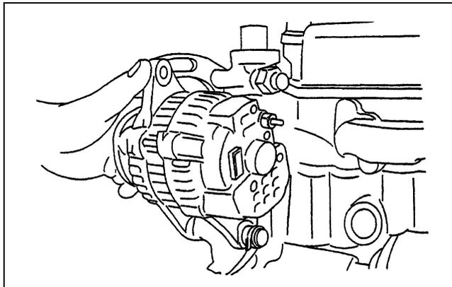
Figure 137 Removing alternator
