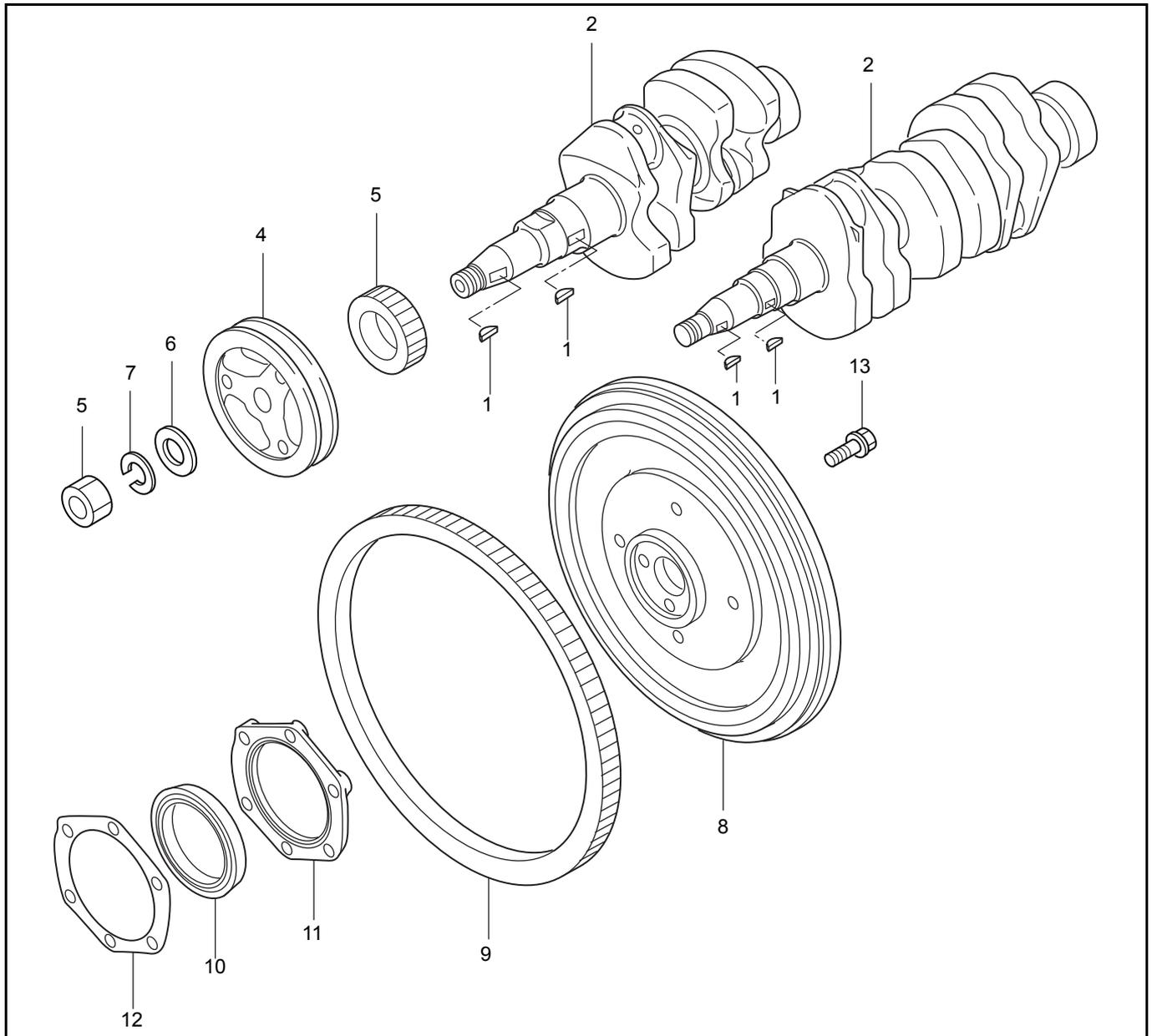
Figure 77 Crankshaft component parts
