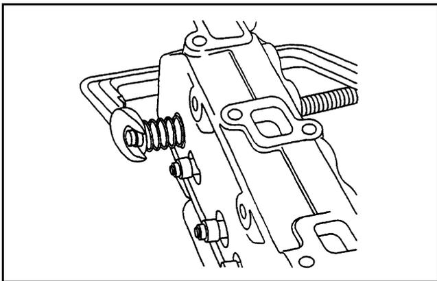
Figure 36 Removing valves
