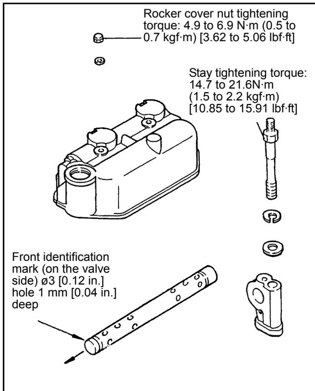
Figure 31 Installing rocker shaft and rocker cover
