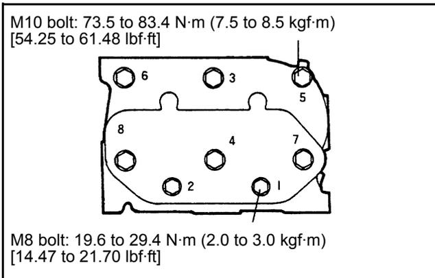
Figure 8 Cylinder head bolt tightening sequence (L2)
