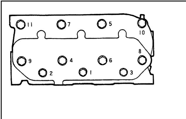
Figure 42 Sequence for tightening cylinder head bolts (L3)
