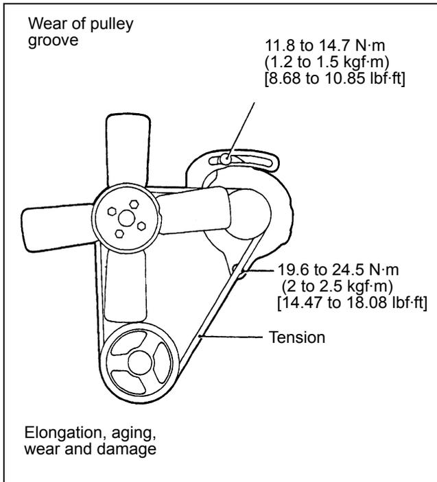
Figure 111 Inspecting fan belt
