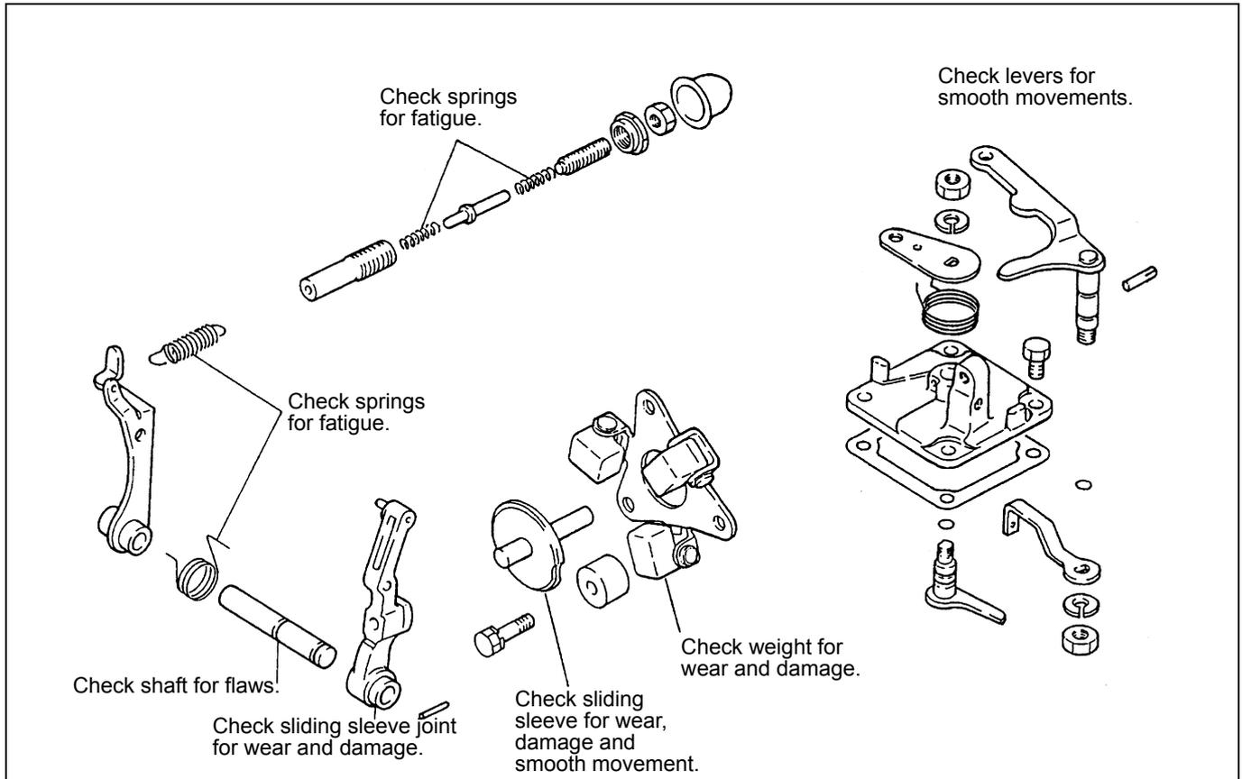
Figure 108 Inspection governor system parts
