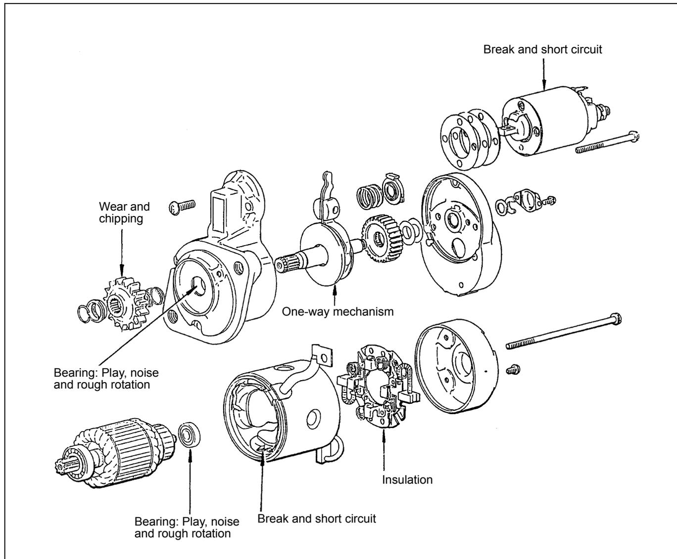
Figure 127 Inspecting starter
