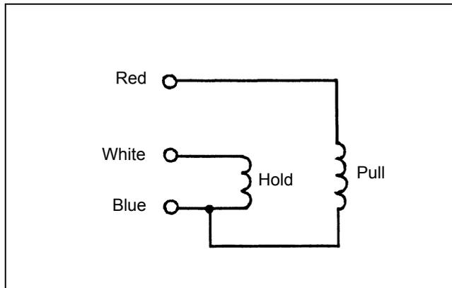
Figure 153 Fuel cutoff solenoid (ETR type) diagram
