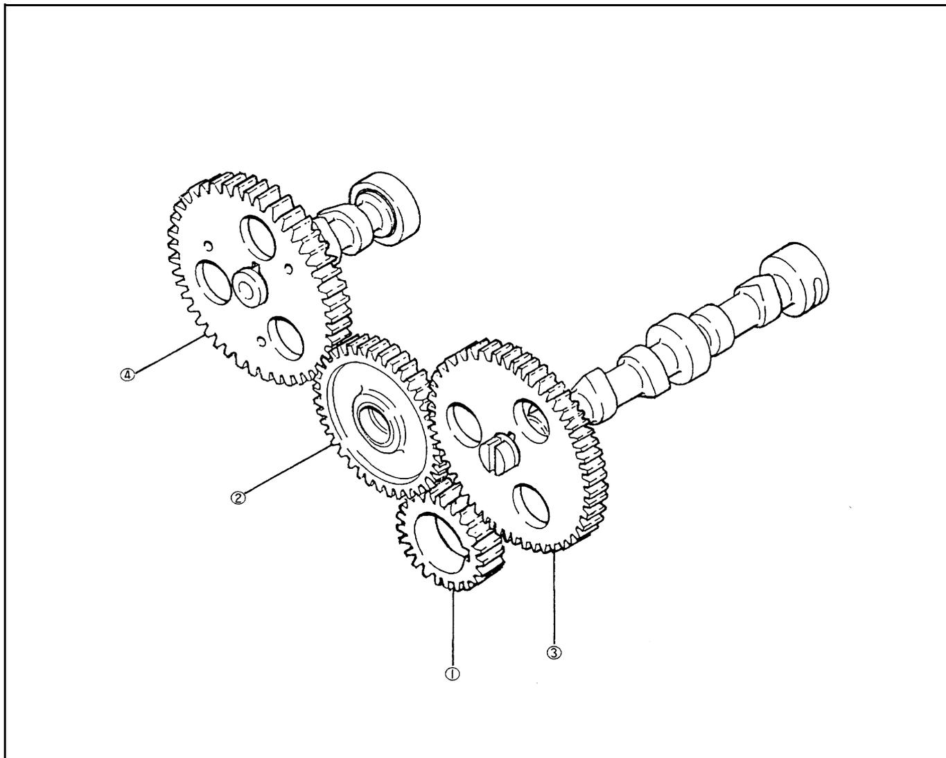
Figure 57 Timing gear component parts
