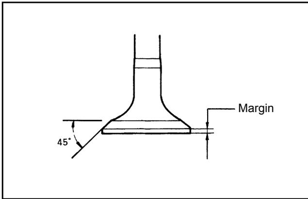
Figure 47 Inspecting valve
