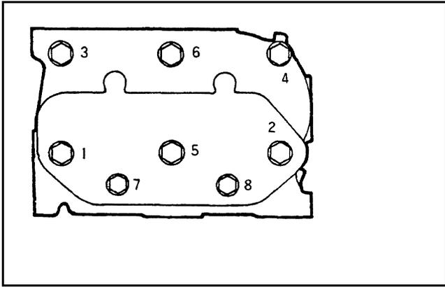
Figure 34 Sequence for loosening cylinder head bolts (L2)
