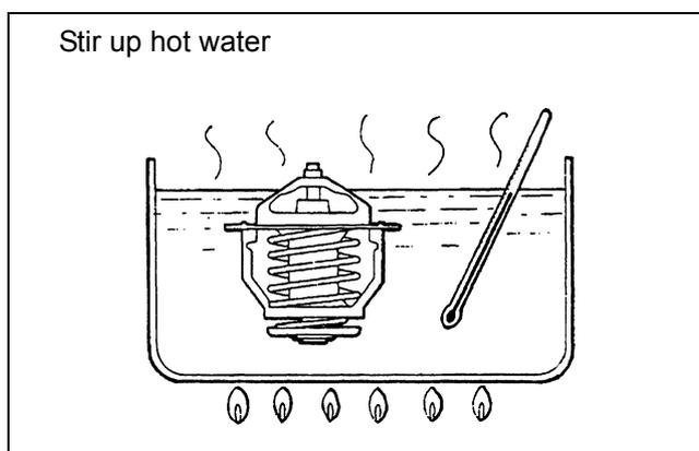
Figure 115 Inspecting thermostat
