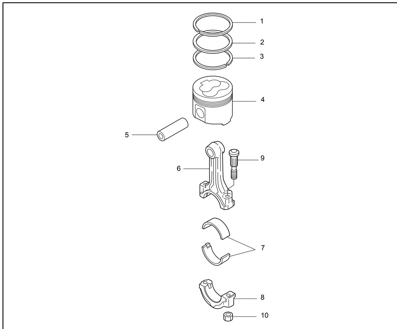
Figure 66 Piston and connecting rod component parts
