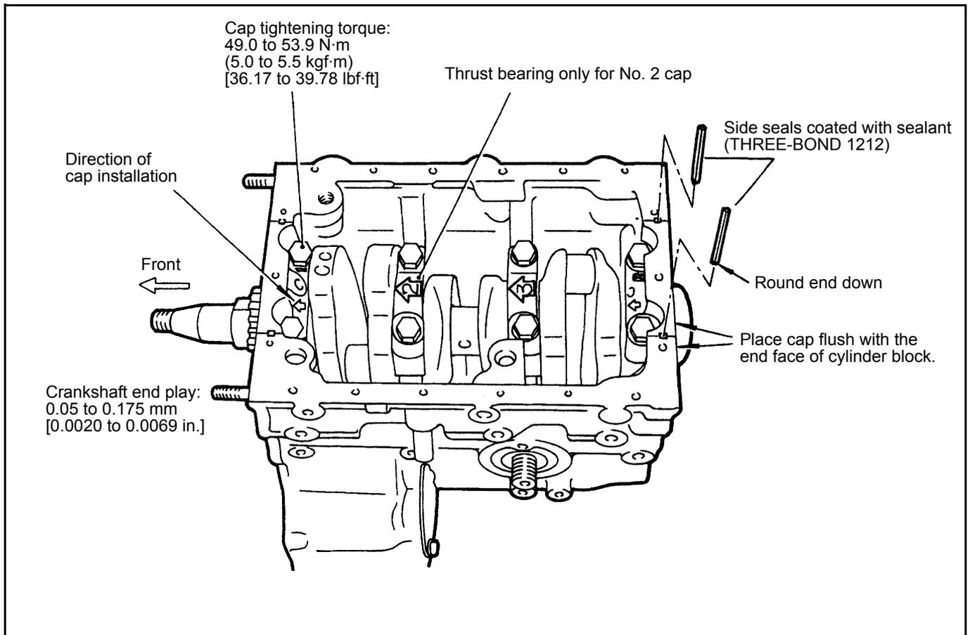
Figure 82 Installation of crankshaft
