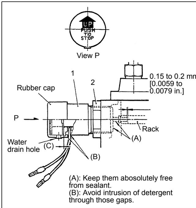
Figure 151 Solenoid installation
