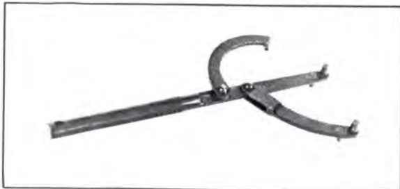
FLYWHEEL HOLDING TOOL Tool No. 90890-01235 OUTIL DE MAINTIEN DE VOLANT Outil No. 90890-01235
