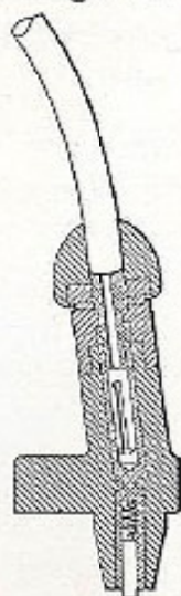
Cross Sectional View of Model EU Terminal
