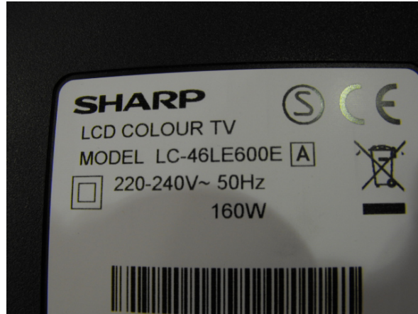
Figure 3: The Model number may be followed by a box containing the Variant letter, the above label shows the [A] variant which must be set in the service mode detailed above along with the 46" in the "INCH SIZE"..
