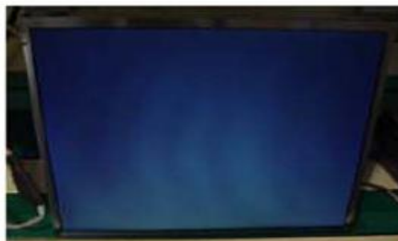
Panel Mura, Light leakage
