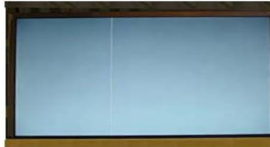
Vertical Line Source TAB IC Defect
