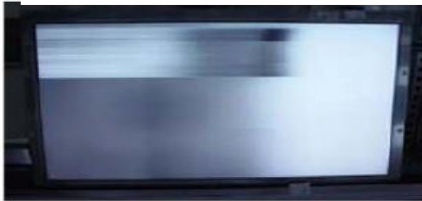
Horizontal Block Gate TAB IC Defect
