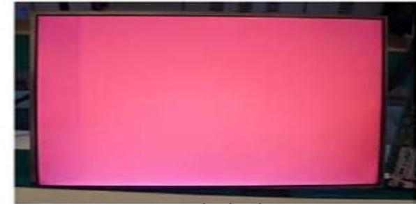
Vertical Block Source TAB IC Defect
