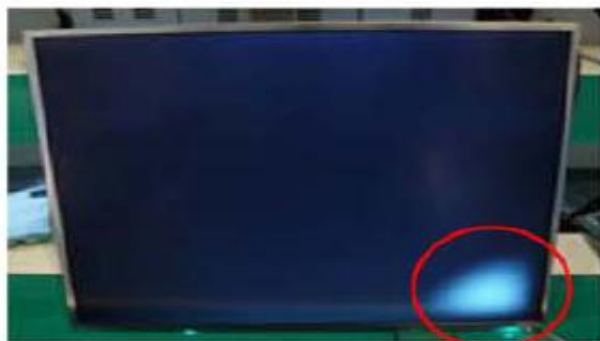
Panel Mura, Light leakage
