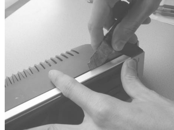
3.Use thin screwdriver to unclench clasp
