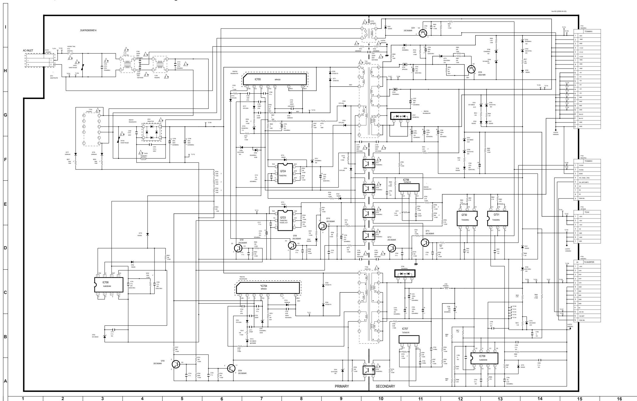
LC-37GD8, LC-37BT8 POWER SUPPLY Unit Diagram
