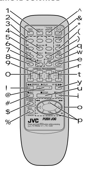
Buttons with a small dot on the left side of the name can also be used to operate your TV while holding down the **TV** button. F pg. 54
