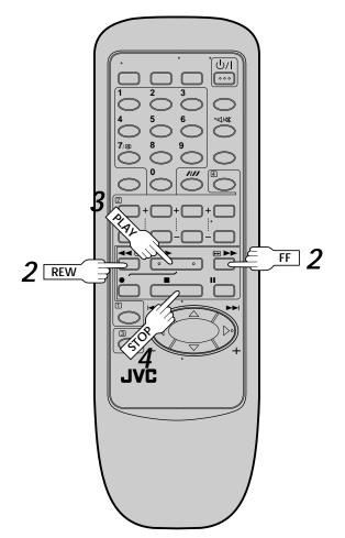
The easiest, most basic operation possible with your video recorder is tape playback. Already-recorded signals on a video tape are read by your video recorder and displayed on your TV just like a TV programme.
