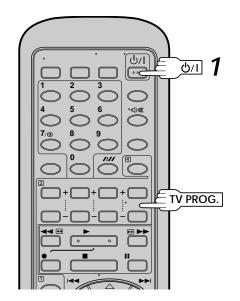
The Auto Set Up function sets the tuner channels, clock and Video Plus+ assigned Guide Program numbers automatically when the U/I button on the recorder/remote is first pressed to power on the recorder after you plug the mains power cord into a mains outlet.
