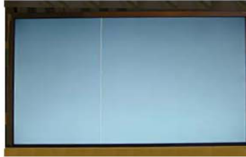
Vertical Line Source TAB IC Defect
