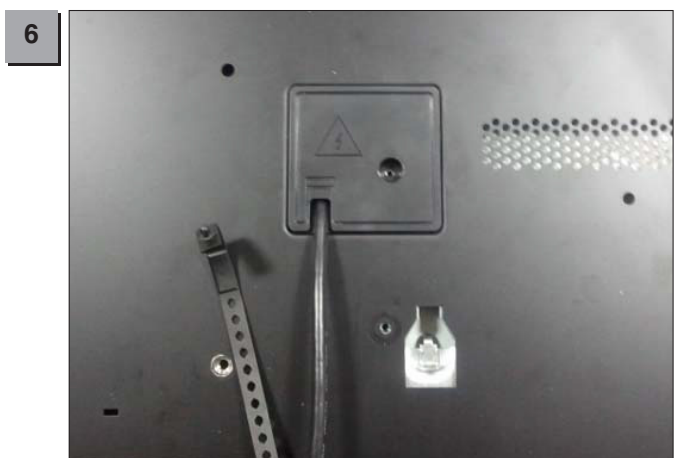
Detach Power cord Cover from the Back cover.
