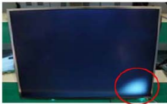
Panel Mura, Light leakage
