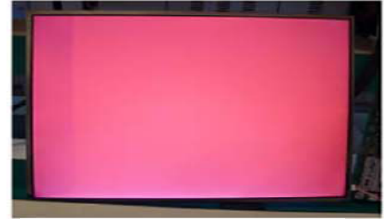
Vertical Block Source TAB IC Defect
