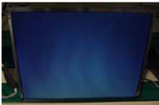
Panel Mura, Light leakage
