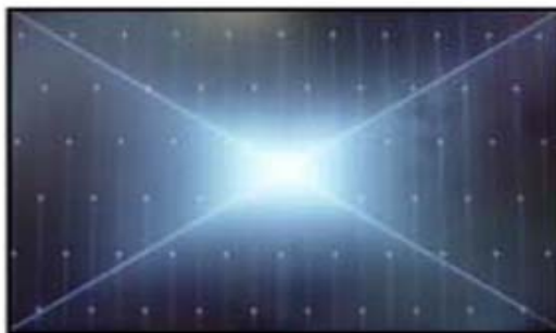
Solder defect, Short/Crack
