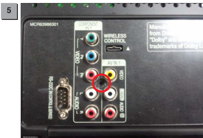
Disassemble 1 screw which bind Main Board and Back cover.
