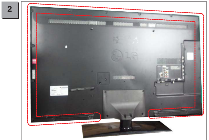
Disassemble 18 screws around the 4 edges of set after separation Stand Assembly.
