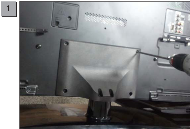
Loosen 4 screws that bind Stand Assembly and set.
