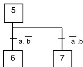
EXAMPLE 1 : The exclusion between the sequences is achieved by the logical exclusion of the two receptivities. If a and b are simultaneously true when step 5 is active , no transition may be cleared.
