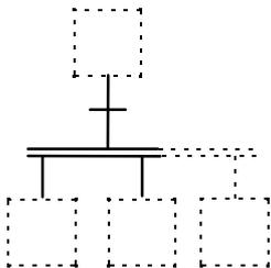
The synchronization symbol N° 18 is used in this structure to indicate the simultaneous activity of several sequences from one or several steps.
