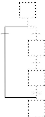
Particular case of selection of sequences, which allows a complete sequence or one or several steps of the sequence to be skipped, when, for example, the actions associated to these steps become unnecessary.
