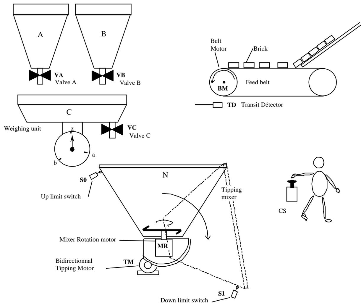
**Figure B1 - Configuration diagram of weighing-mixing system**
