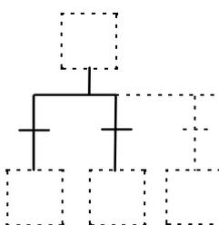
The selection of sequences shows a choice of evolution between several sequences starting from one or several steps. This structure is represented by as many simultaneously enabled transitions as possible evolutions.
