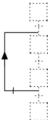
Particular case of selection of sequences, which enables a sequence to be repeated until, for example, an established condition is satisfied.
