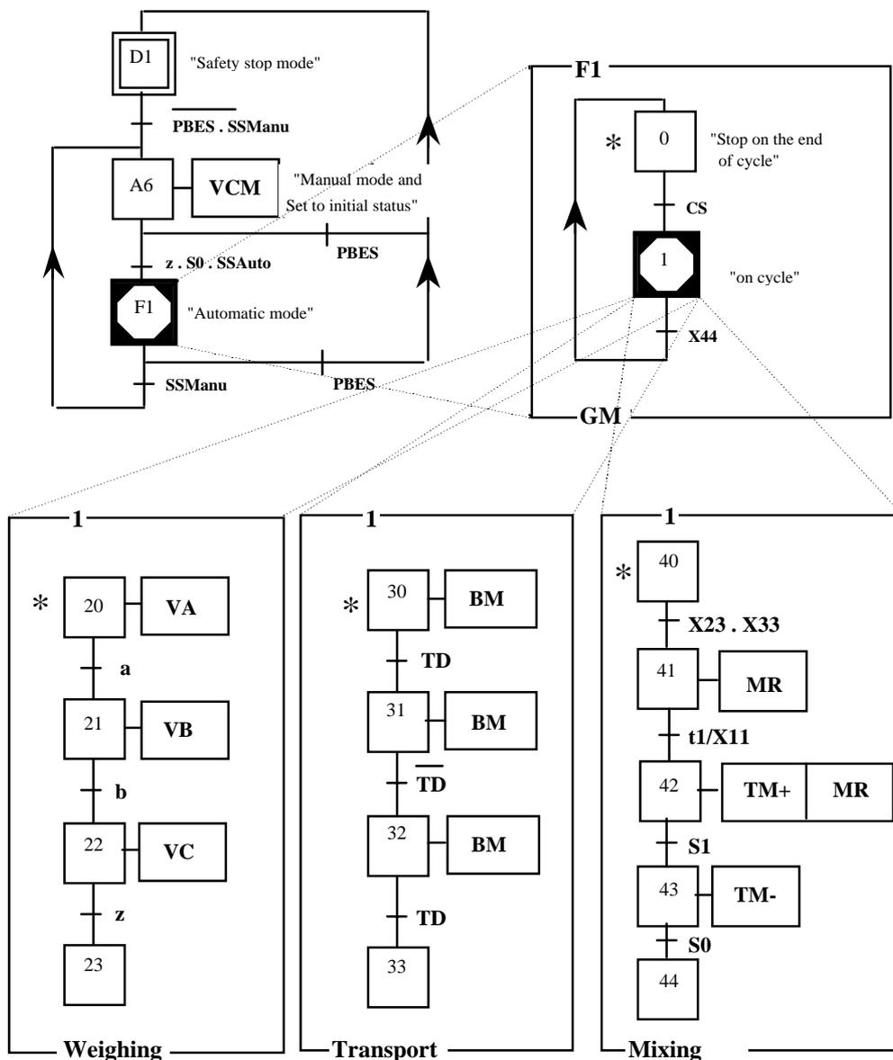
**Figure B6 - Structure with operating modes using enclosing steps :**
