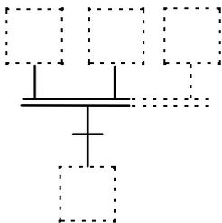
The synchronization symbol N° 18 is used in this structure to indicate the waiting for preceding sequences to end before activating the succeeding one.
