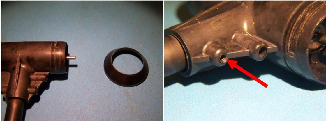
With the retaining screw loosened, carefully feed the cable up the arm whilst pulling on the head unit. The two should separate.
