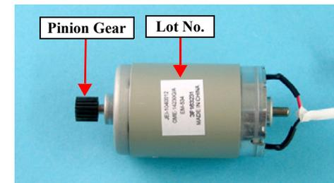
Figure 4-32. Installing PF Motor
