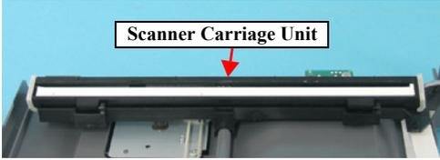
An image showing the scanner carriage unit with a red arrow pointing to it and a label 'Scanner Carriage Unit' above the arrow.                                                      | 1. Replace the Scanner Carriage Unit with a new one.              |
