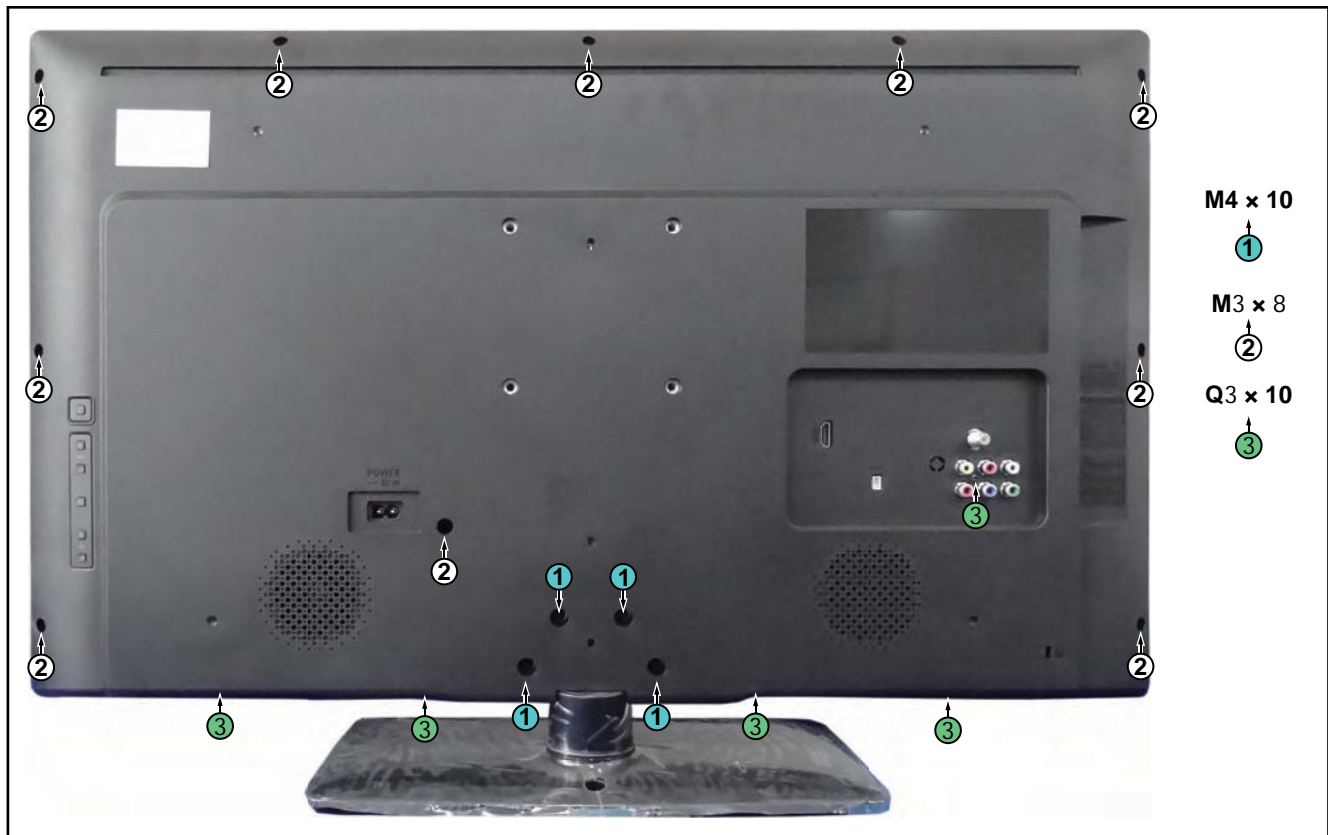
Figure 4-4 Rear cover removal
