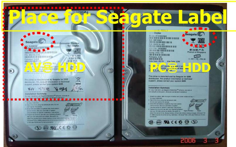
SVC: Replace HDD for PC with low-noise HDD for AV.
