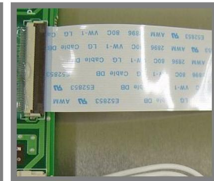
① **Replace Y or Z B/D : Most maldischarge is caused by Y or Z.**
