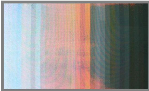
**Mal discharge by board defect**
