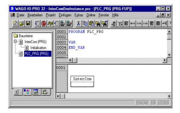
Existing programs can easily expanding they are functionality for data exchange by adding this program, and call the program In the PLC PRG.
