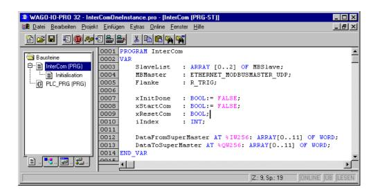
The necessary parameters for the function block are stored in the "SlaveList".. This "SlaveList" is an array of type "MBSlave" and will be initialized on program start with the action "InterCom.Initialsation".
