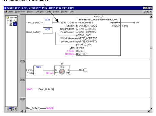
The Timeout value is directly written into the function block. This is the maximum time the master waits for an answer of the slave. If the slave does not respond during that time, the error code will be written into the error word.
