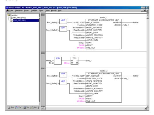
The ETHERNET\_MODBUSMASTER\_TCP function blocks have to be programmed identically.
