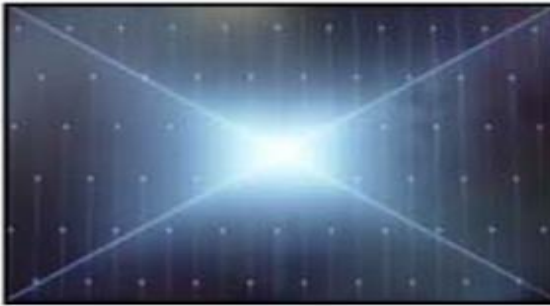
Solder defect, Short/Crack
