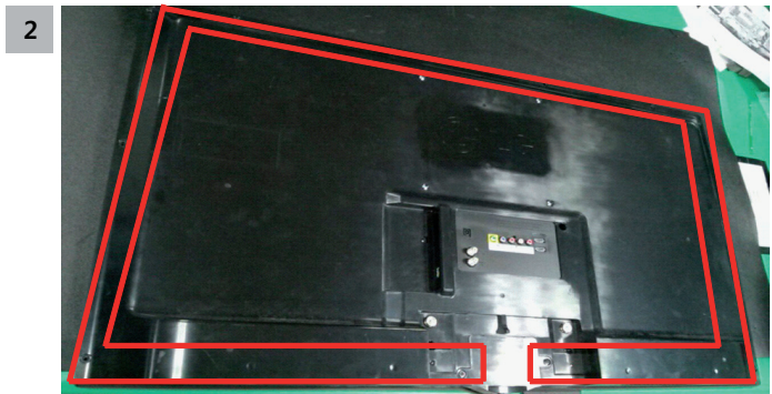
Disassemble 13 screws around the 4 edges of set after Separation Stand Ass'y
