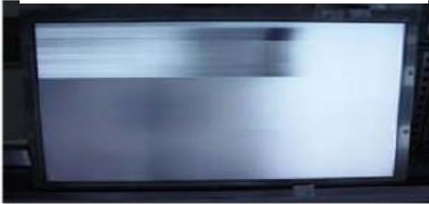
Horizontal Block Gate TAB IC Defect
