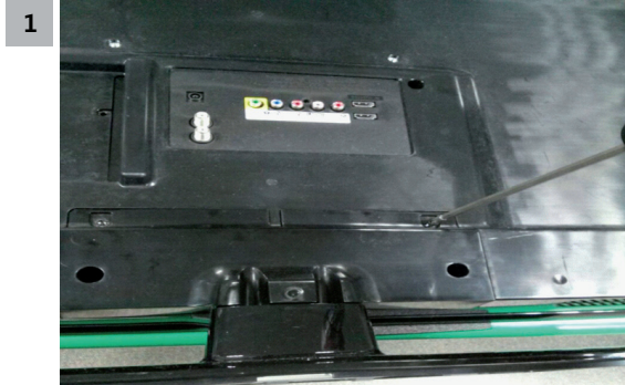
Loosen 4 screws that bind Stand Ass'y and set
