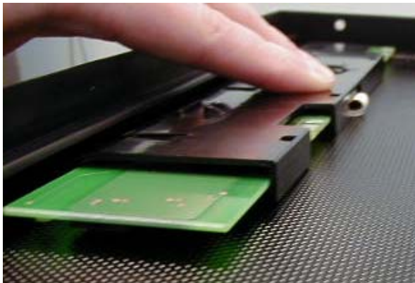
(32) Turn down the electronic with displays onto the glass side, press the carrier flatly to the glass lower side and let it lock in. For assembly press the locking slightly to the bottom.
