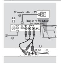
Helpful hint: Before making or changing any connections, make sure that all the devices are disconnected from the power outlet.
