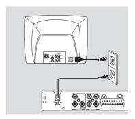
After everything is connected properly, plug in the AC power cord to the power outlet.
