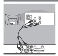
Use the composite video cable (yellow) to connect the DVD player's VIDEO(CVBS) jack to the video input jack(or labelled as A/V in,Video In or Composite) on the TV(cable not supplied). To hear the sound of this DVD player through your TV, use the audio cables(white/red)to connect AUDIO OUT(L/R)jacks of the DVD player to corresponding AUDIO IN jacks on the TV(cable not supplied).
