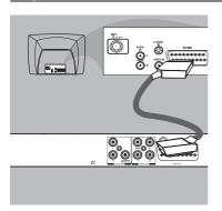
Use the scart cable to connect the DVD SCART OUT to the corresponding scart input socket on the TV (cable not supplied).
